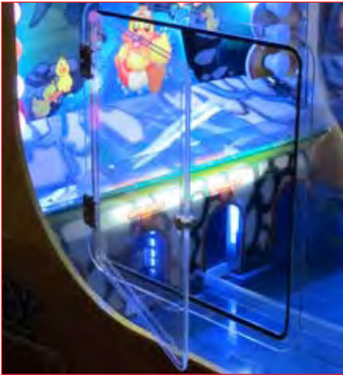
Maintenance doors Service doors on both sides of the clear plexi for easy access to the playfield
